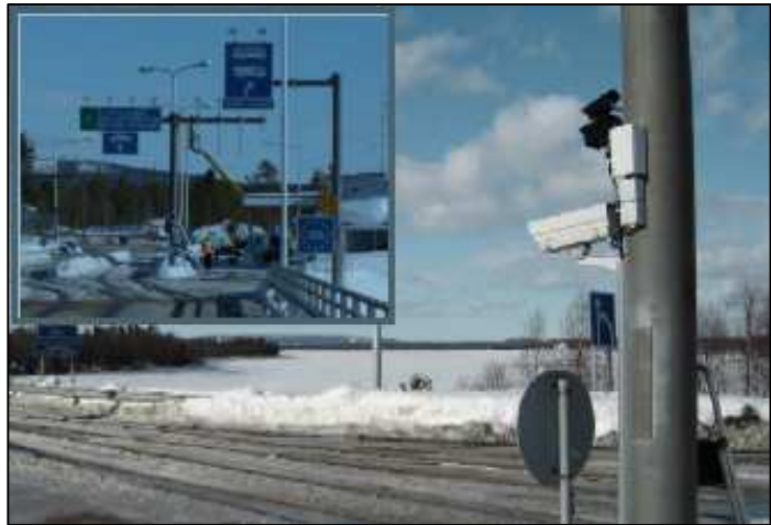
License plate capture cameras can be used to improve border security and operations. The camera system above provides high-resolution license plate imaging to intelligent software at the Sweden-Finland border.
