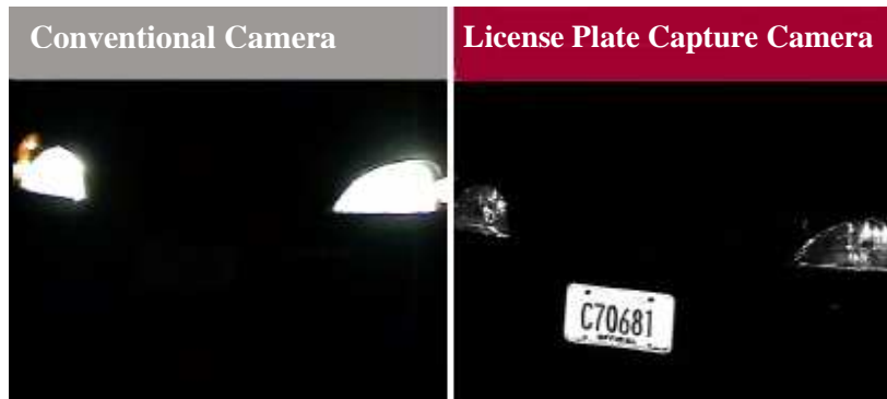
Overcoming the problems of headlight glare and low lighting, cameras specially designed for license plate capture such as Extreme CCTV's REG ® (right) are capable of delivering highly resolved images in subzero temperatures.
