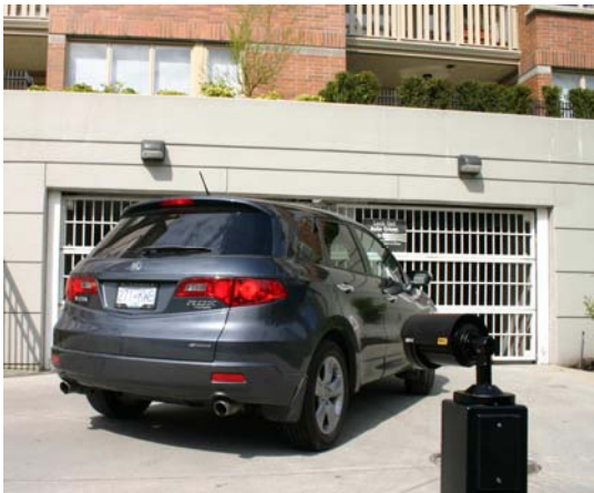
License plate capture can be used for vehicle surveillance and access control into and out of a gated community, university campus or parking garage. The camera can also be integrated with video analytics to create a license plate recognition system.
